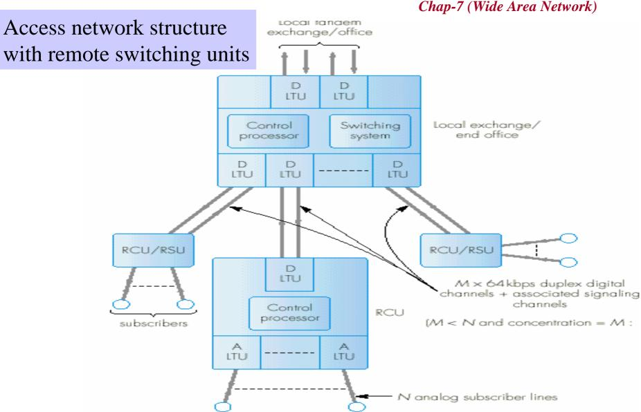
RSU = remote switching unit RCU = remote concentrator unit D/A LTU = digital/analog line termination unit
