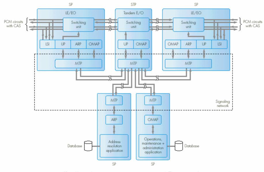
ARP = address resolution part UP = user part OMAP = operations, maintenance, and administration part LSI = local signaling interface MTP = message transfer part SP = signaling point STP = signaling transfer point
