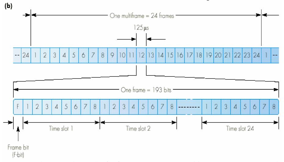
Note: Frame alignment signal (FAS) = F-bits from frames 4, 8, 12, 16, 20, 24 and these are set to 001011 respectively
